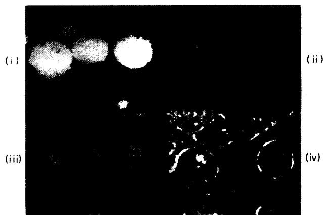
Fig. 3. XRMA scanning picture of Si1 . Pd (iii) and Cl (ii) distribution appears to be fairly regular throughout the silica beads cross sections. Silicon distribution (i) and SEM (iv) are also presented.
